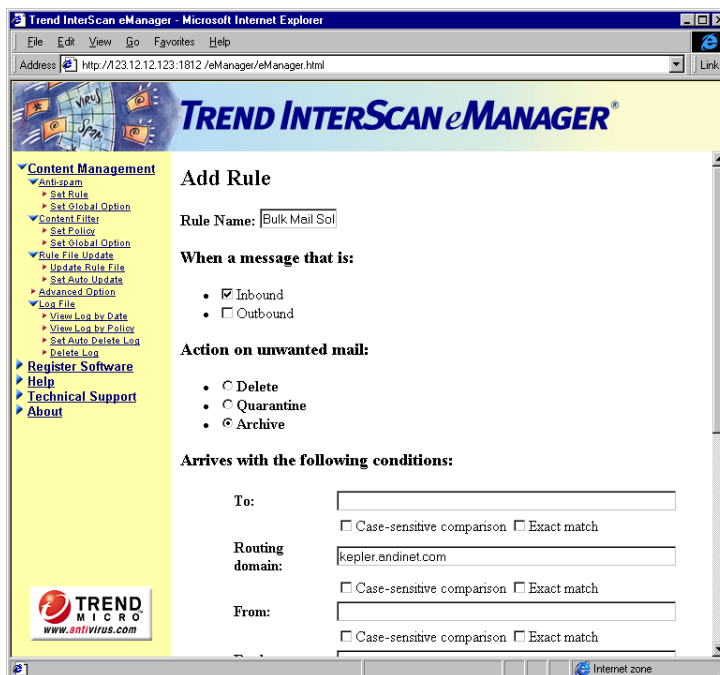
FIGURE 2-3. The Add Rule page showing the routing domain used to block spam.
